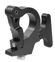
The Slim-Claw will fasten to both 1-1/2" pipe (1.90" OD) and 2" OD truss tube. The Slim Claw has a 3-1/2" T-handle, so no tools are required to fasten to the pipe. Comes with 1" x 1/2"-13 TPI Grade 5 fastener and 1" diameter Belleville Spring washer.
